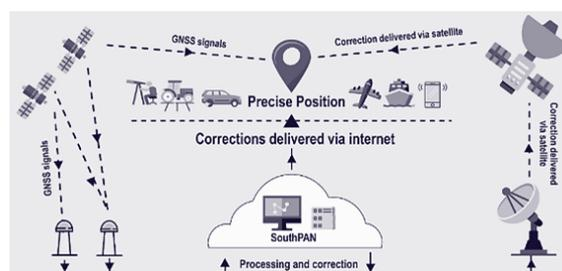
Mining also benefits from 3 cm precision positioning provided by RTK systems and the CORS network. The **National Positioning Infrastructure Capability program** provides 3cm accuracy satellite positioning that is of value to the mining sector for activities such as monitoring tailings dams and precise positioning in a range of activities including management of mining operations to protect environmentally and culturally sensitive areas, management of stockpiles and rehabilitation activities.
